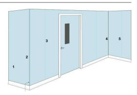
Material: Extruded semi-rigid PVCu and aluminium
